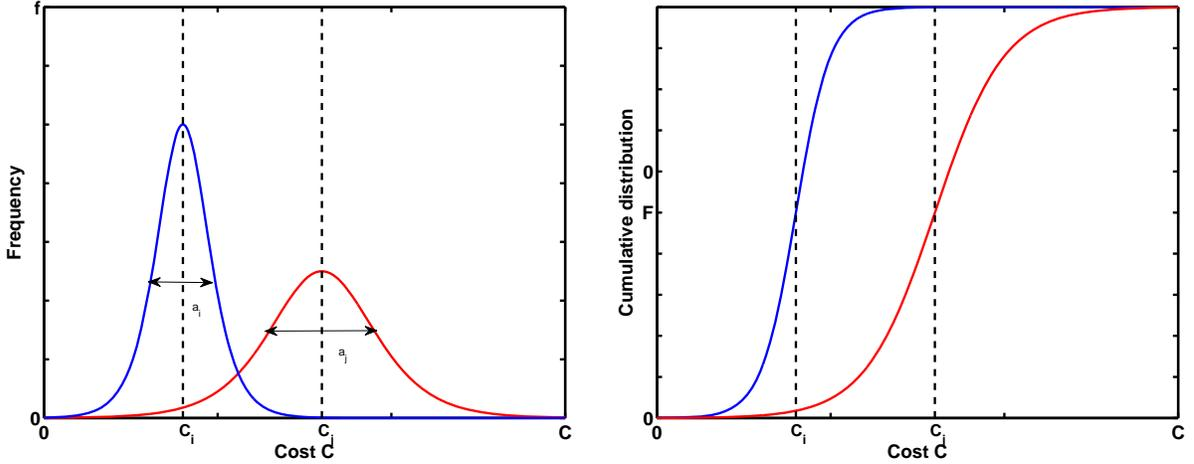
Figure 1: *Left* Distribution of costs for two different energy technologies, denoted  $i$  and  $j$ . These have median costs  $C_i, C_j$  and widths  $a_i, a_j$ . *Right* Cumulative cost distributions. These correspond to the fraction of potential units with cost below threshold  $C$ .
