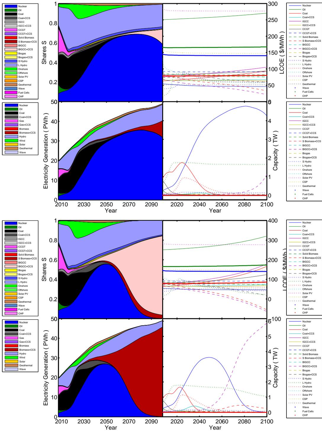
Figure 10: Carbon price increasing by 1%/y (top) and 2% per year (bottom) using a discount rate of 5%.
