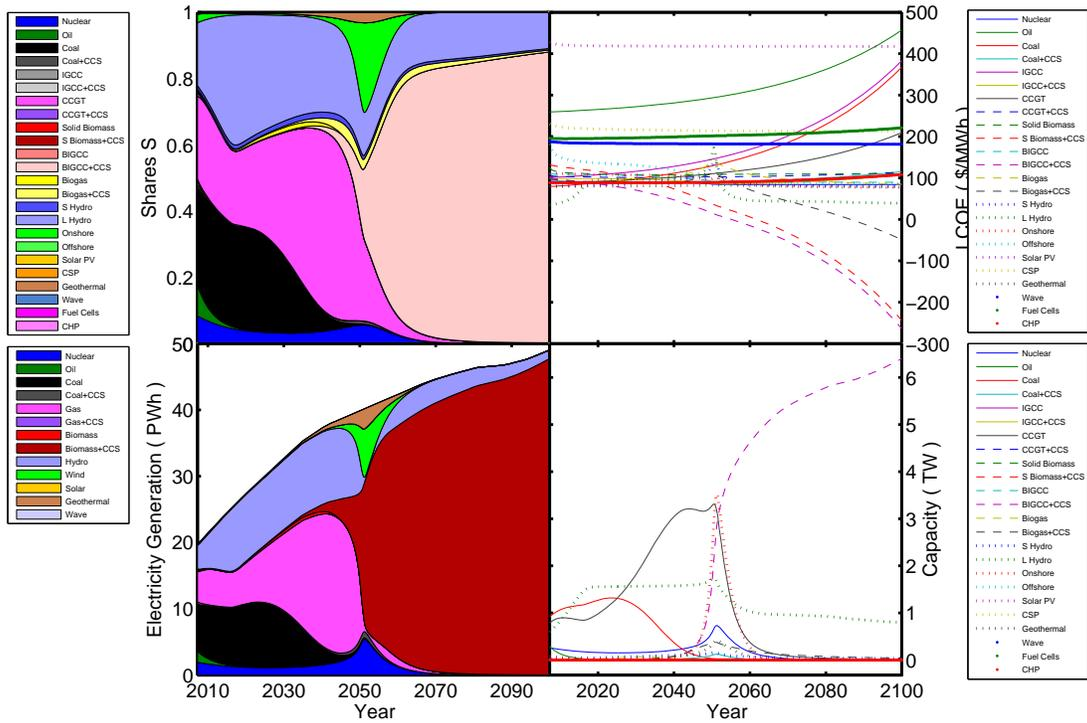
Figure 13: Carbon price increasing at a rate of 3%/y, and a discount rate of 10%.
