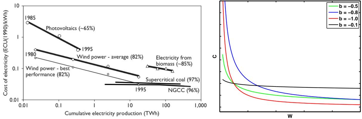
Figure 3: *Left* Technological learning curves for several electricity generation technologies, calculated by the IEA (IEA, 2000). Progress rates are given in brackets. The exponents  $b_i$  are related to the progress rates  $a_i$  through  $b_i = \ln(1 - a_i)/\ln(2)$ . *Right* Learning curves plotted on a linear scale for various exponents.
