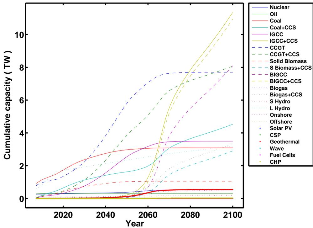
Figure 16: *Top* New capacity. *Bottom* Cumulative capacity.
